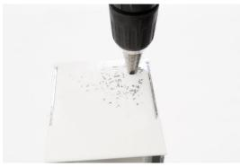
Use a larger drill or step drill bit to expand the hole to the size you need.
