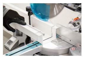
Fasten and cut the length of the box to suit the structural opening length.
