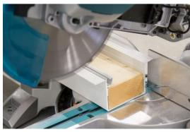
To support the profiles, especially when using smaller saws, a piece of timber can be used.
